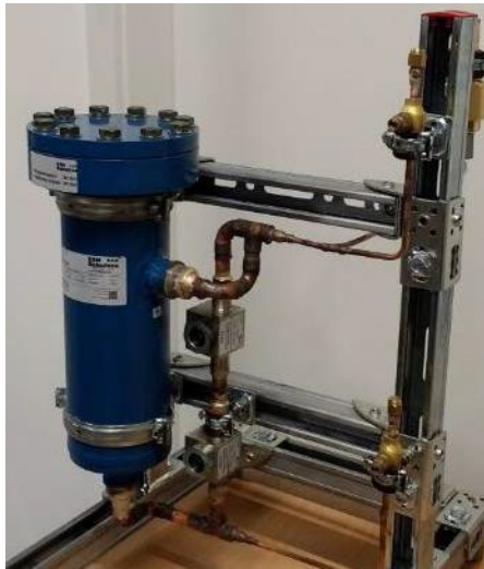
Figure 2: Autoclave for the loose storage of test objects in hydrogen
