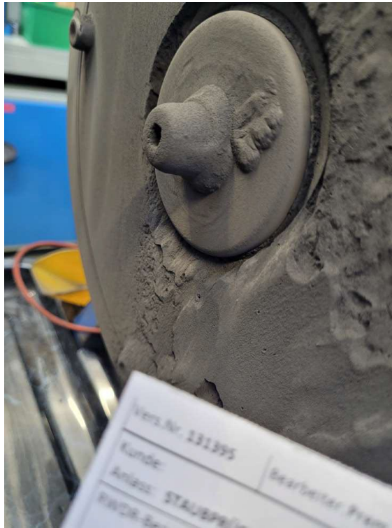
Figure 6: Sealing tests – test of a soft seal under contamination of a soft seal; source: Freudenberg sealing technologies
