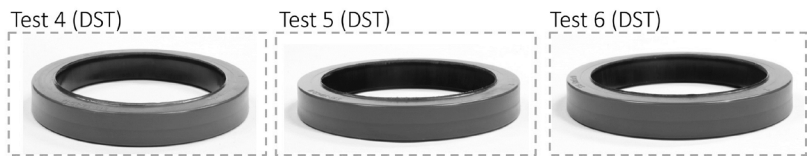
Figure 7: Seal pictures after testing from Test 4 (DST) to Test 6 (DST)
