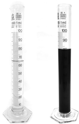
Figure 2: Degradation of the hydraulic oil results in a darkening of oil
