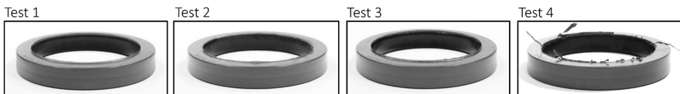
Figure 5: Seal pictures after testing with untreated oil
