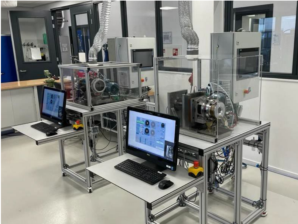
Figure 5: High-speed test rigs for seal performance testing. Testing capabilities: High speed testing up to 50.000 rpm, High temperature up to 180°C, Controlled pressure/vacuum up to 100 mbar +/- 0.2 mbar, oil bath or oil mist, pumping and leakage (visual, mass).
