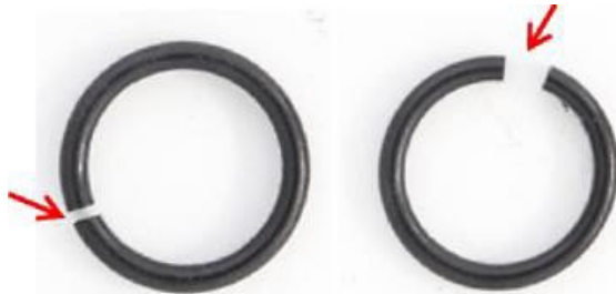
Figure 3: O-ring: hardening due to high thermal load
