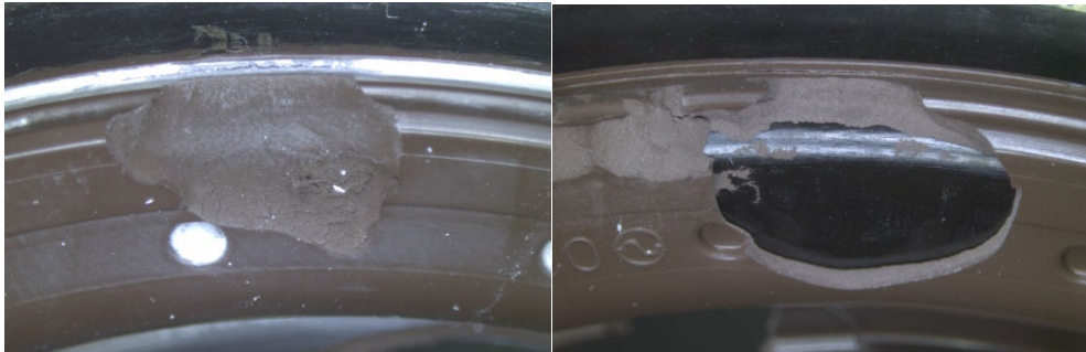
Figure 3: Adhesion test result: good adhesion (left) and poor adhesion (right) [4]
