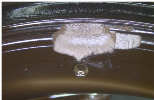
Figure 4: Adhesion test after 1000 h storage in gear oil at 150° [4]
