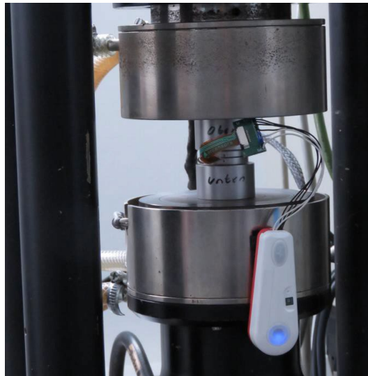
Figure 5: Test setup to validate the foil sensor
