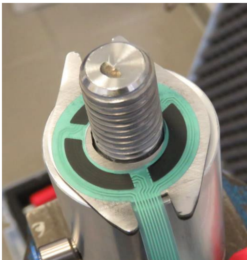
Figure 3: Foil sensor with three pads for alignment measurements
