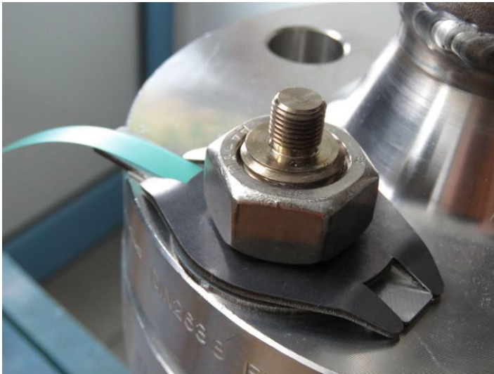
Figure 2: Washer with integrated foil sensor
