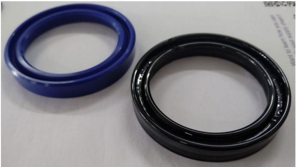
Figure 4: Injection molded XT200 vs 2 Wall Print
