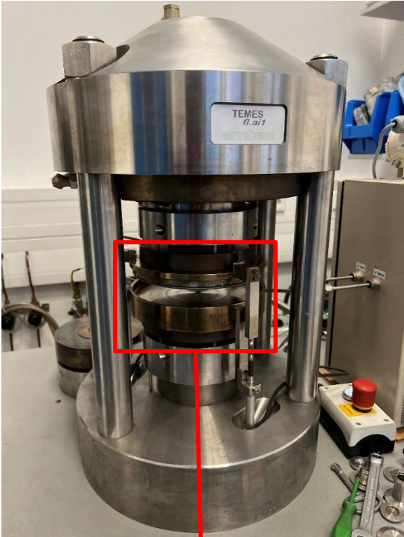
Figure 6: Experimental setup for carrying out the compression tests
