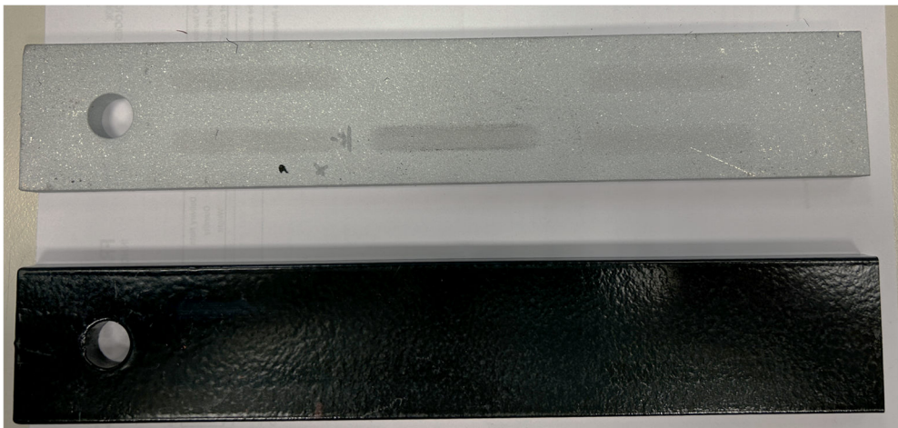
Figure 4: Coated test specimen – white metallized coating (top) and black (bottom)
