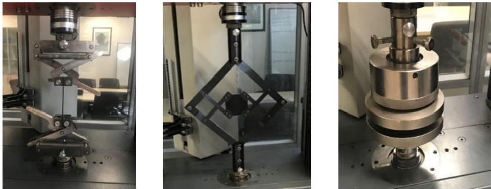
Figure 4. Tests (a) Uniaxial Tensile (b) Biaxial Tensile (c) Compression
