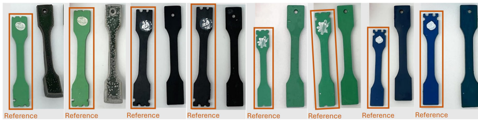
Figure 1: Visual representation of the volume change of samples right after immersion for 1,512 h at +80 °C and after redrying in a vacuum oven. Left to right: EPDM 1, EPDM 2, FKM 1, FKM 2.
