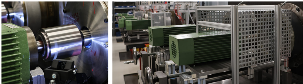
Figure 4: Images of the endurance seal test rigs. In the left image, the camera observing leakage is visible
