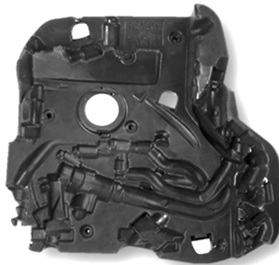
Figure 3. EPDM foam cover can collect salt water and expand period of corrosion attack
