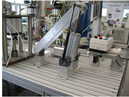
Figure 4: seal testing for gas spring applications
