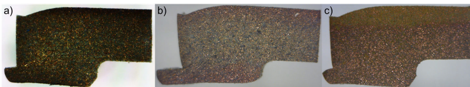
Figure 9: Seal cross-sections of three seals made of a) virgin T46, b) T46_R25, and c) T46_R66 (PTFE compound with 66 wt.% bronze-filled PTFE repro and virgin PTFE).
