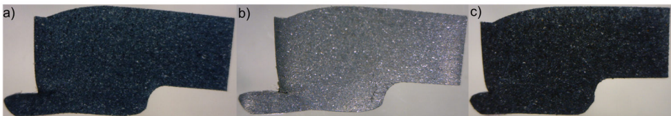
Figure 12: Seal cross-sections of the three seals made of a) virgin M12, b) M12_R15, and c) M12_PR15.
