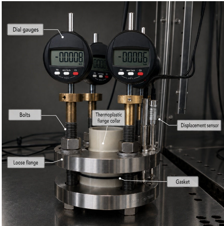
Figure 2: Design of the measurement cell used
