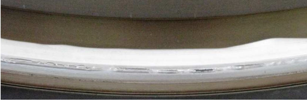
Fig. 6: Delamination of silver plating after thermal cycles
