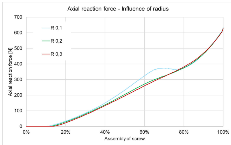
Figure 14: Influence of the edge radius on the axial reaction force during assembly
